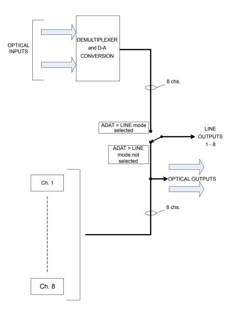
This mode allows you to use the Clarett+ OctoPre to connect an 8-channel ADAT format output (from a DAW, for example) to a set of analogue inputs. For example, you can send the channels from your DAW to outboard equipment to use as part of your mixing process.
