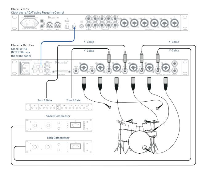
When recording acoustic drums, you can use dynamics control in various ways to get the sound you're after. Compression is often added to kick and snare drums to thicken the sound, while noise gates are effective on toms to minimise spillage between the drum mics.
