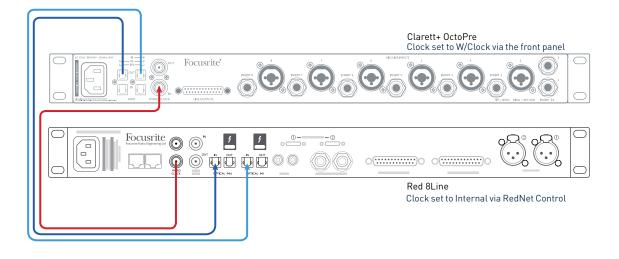
This example shows a similar setup as Example 2, but using a Focusrite Red 8Line audio interface running at a sample rate of 96 kHz ("SMUX-II" mode). Both units must be set to 96kHz; you need two optical cables, carrying four channels of audio each. The Red 8Line is the sync leader.
