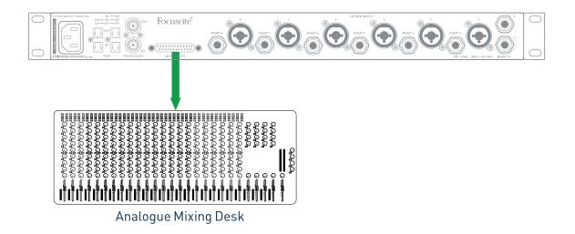
This setup uses the Clarett+ OctoPre's mic preamplifiers and AIR mode to provide a high quality "front end" for an analogue mixing desk. Use an 8-way loom to connect the OctoPre's LINE OUT socket to eight line inputs on the mixing desk; this will need a 25-way D-sub on one end and eight connectors appropriate to the desk's line inputs on the other. (Pre-made looms are available from professional audio suppliers).
