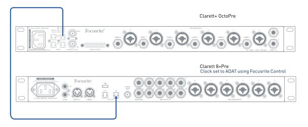
Here the **OPTICAL OUT** on the Clarett+ OctoPre is connected to **OPTICAL IN** on a Focusrite Clarett+ 8Pre audio interface with a single optical cable. Both units are running at 44.1 kHz sample rate. The OctoPre's clock source is set to INTERNAL, and the 8Pre is synchronised to it because its clock source is set to ADAT (via Focusrite Control).
