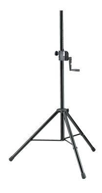
A high quality steel speaker stand with plastic clamps for professional use. Infinitely variable height adjustment with a hand crank and push button system which prevents an uncontrolled reverse motion. There is an additional locking screw for extra safety. Extension tube diameter 35 mm, suitable for speakers and lighting crossbars with an integrated M10 thread connector.
