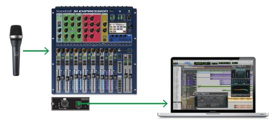
The MADI-USB Combo card also enables multi-track recording and playback. Standard mic/line input sources can be recorded through the Si series console via the card to a DAW or similar. This simple yet powerful solution is suitable for recording live gigs but is equally at home in the studio.
