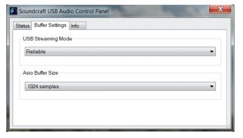
Recommended buffer size will vary depending on application, however higher buffer sizes should be used when monitoring from the DAW is not necessary. For most live recording applications, a standard buffer size of 1024 samples is enough to ensure reliable operation and clean audio.
