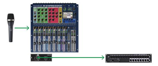
MADI is a standard protocol on all Soundcraft Stageboxes including the Compact Stagebox and Vi Stagebox. The connection to a Stagebox works exactly the same for all Soundcraft consoles and Stageboxes.
