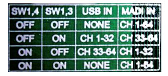
SW1.4 and SW1.3 is short for switches 3 and 4 respectively on the first dipswitch on the option card.
