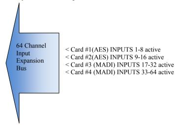
This configuration uses all four slots found in an Si3 / Si2 but no two cards are trying to route to the same bus.
