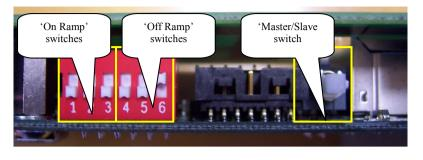
The master / slave status determines the clock source for the BLU link network.
