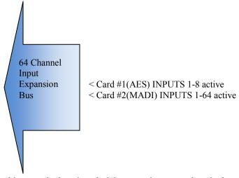
In this example there is a clash between the two cards as both are trying to 'route' to buses 1-8 and the conflict must be resolved by resetting of the routing dip switches on one or other of the cards.
