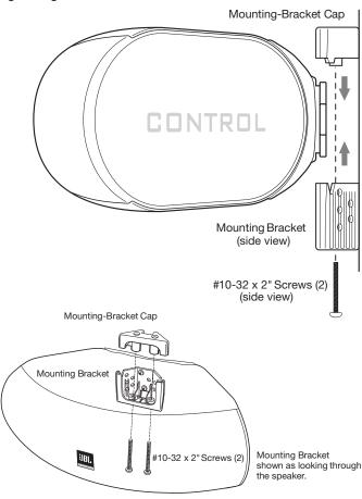
6. To orient the JBL logo into the correct position, pull the JBL logo slightly outward from the speaker grille and rotate. The JBL logo is held in place by a spring. Peel the adhesive cover off the mounting-bracket cover and attach to the top and bottom of the mounting accomply.
