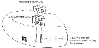
6. To orient the JBL logo into the correct position, pull the JBL logo slightly outward from the speaker grille and rotate. The JBL logo is held in place by a spring. Peel the adhesive cover off the mounting-bracket cover and attach to the top and bottom of the mounting assembly.
