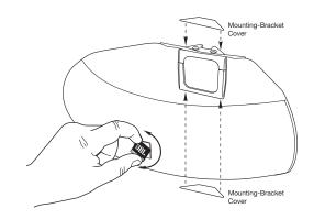
7. VERTICAL BRACKET ORIENTATION —Regardless of whether you choose a vertical or horizontal orientation for the speaker, when mounting the JBL Control CRV speaker to a single wall surface, you should always install the wall-mounting **bracket** in a vertical orientation.
