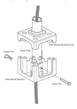
4. The pole-mount bracket can now hold the weight of the speakers.
