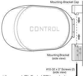
6. Rest the second JBL Control CRV speaker's rear flange in the mounting bracket, as shown. Secure the mounting bracket cap with two #10-32 x 2" (M5 51 mm) screws through the bottom of the mounting bracket.
