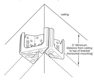
2. Attach the mounting bracket to the wall. Be sure to use appropriate anchors.
