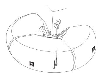
8. To orient the JBL logo into the correct position, pull the JBL logo slightly outward from the speaker grille and rotate. The JBL logo is held in place by a spring. Peel the adhesive cover off the mounting-bracket cover and attach to the top and bottom of the mounting assembly.
