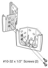
When deciding upon a location for the JBL Control CRV speaker, take care NOT to install the mounting bracket closer than 3" (7.6 cm) (horizontal) and 8-1/2" (21.5 cm) (vertical) to the ceiling. Any closer than the minimum measurements will not allow the clearance needed to position and slide the JBL Control CRV speaker into the mounting bracket.
