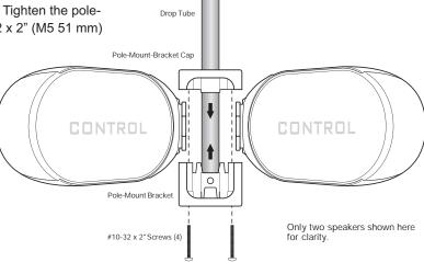
4. Place the pole-mount-bracket cover over the bottom visible mounting bracket by snapping it into place.
