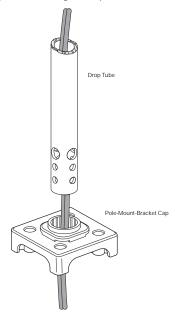
2A. Slide the pole-mount bracket up onto the drop tube, aligning the pinholes on the bracket with those on the drop tube.
