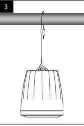
3. With speaker supported, snap main support hook hanger onto the center hole in the top bracket of the speaker. Adjust to proper height by pulling cable through either end of Gripple.
