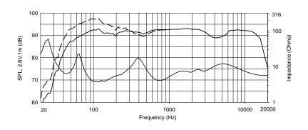
Frequency Response, on axis in half-space  $(2\pi, dotted$  line) and full space  $(4\pi, solid line)$  at thru  $(8\Omega)$  setting, Input Impedance.
