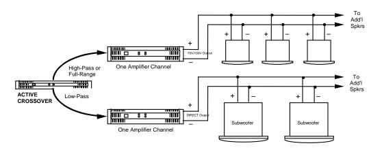
Note: JBL MPC-T amplifiers have the ability to simultaneously drive a 70V/100V line from one channel and low impedance speakers on the other channel, such as shown in diagram.
