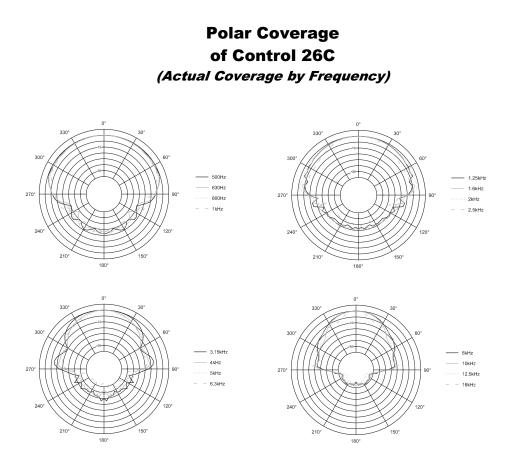
**Single Speaker Coverage** – The coverage area of a single speaker depends on the distance of the speaker from the listener, which depends upon the ceiling height and the listening height (seated vs. standing). The following chart assumes a 4 ft (1.2 m) listening plane and averages coverage over the 500 Hz to 8 kHz range:
