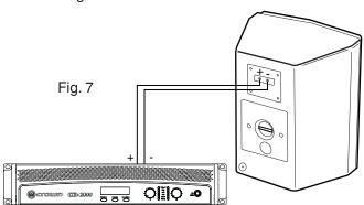
Before turning on the amplifier, make sure the speaker tap switch is set to the proper selection. Sending a 70/100V feed to the Control 25AV-LS in its bypass mode may result in permanent damage to the loudspeaker.
