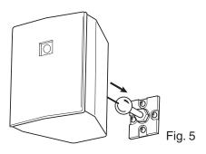
6. Tighten the clamp just enough to hold the speaker while it is positioned in its desired orientation. When the speaker is in the desired direction, tighten the InvisiBall clamp as shown in Fig. 6 and replace the logo badge.
