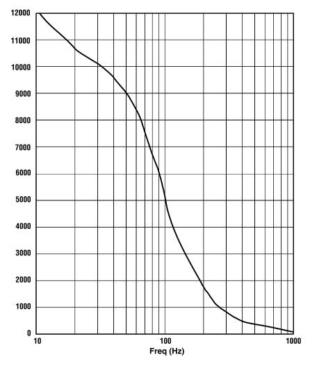
Typical Damping Factor vs. Frequency
