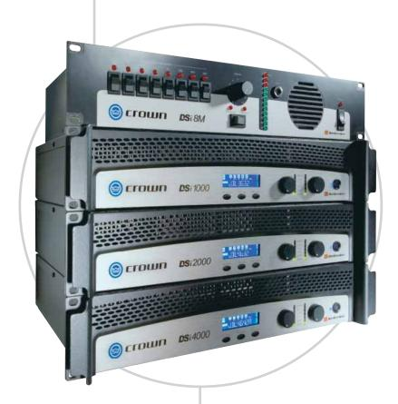
The Crown® DSi Series of power amplifiers provides onboard digital signal processing including crossovers, EQ filters, delay and output limiting. A rear panel HD-15 connector provides easy input/output connectivity between DSi amplifiers and the new DSi 8M System Monitor. All DSi amplifiers are THX® approved.
