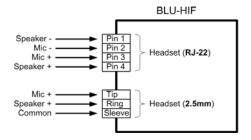
Caution: Do not connect to both jacks simultaneously. Doing so risks damaging the connected devices. Before connecting to either jack, ensure that the internal jumper is set to the appropriate position. By default, the BLU-HIF ships with the jumper in the Headset **RJ-22** jack position.
