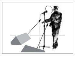
Fig. 2: Microphone placement for maximum gain before feedback.
