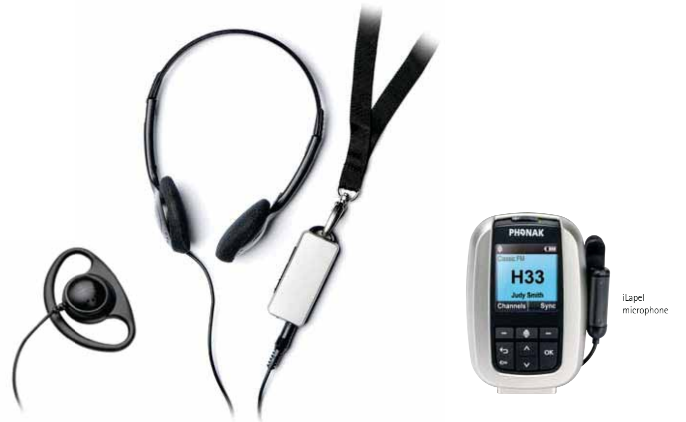
Robust inspiro transmitter microphone (worn by guide)
