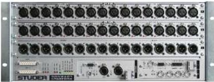
The Compact Stagebox adds a cost effective expansion option, offering a high density of I/O connections in only 4U of rack space. The modular unit is fully configurable but is offered with a standard configuration of 2 x HQ mic/line input modules, line output module, D21m MADI HD RJ45 card and blank panels for the D21m slots.
