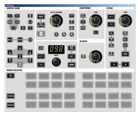
A GUI monitoring page mirrors all monitoring controls of a real Vista desk (see above). This page is operated from the touch screen and can be called up by a physical key on the controller. For talkback, a gooseneck mic can be plugged into an XLR socket on the face plate. Its signal is fed through to an XLR socket at the rear.
